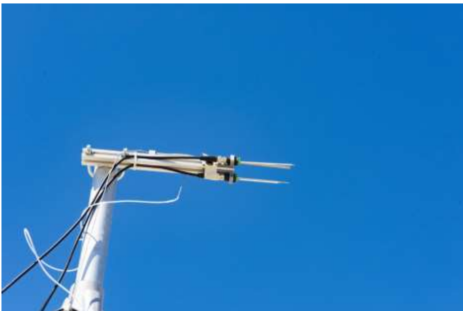
Figure 2: One station of the set-up deployed at Utah's SLTEST facility. An NSTAP, a TNSTAP, a pitot tube, and a thermocouple are mounted.
