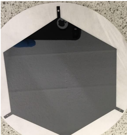
Figure 1: Example of a silicon wafer fabricated at the PRISM cleanroom used for mechanical validation of prototype designs of the Simons Observatory detector and readout wafer stack.
