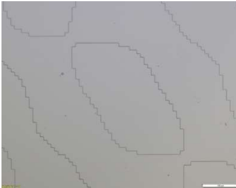
Figure 1: Diffractive Element Optics (DOE) on a glass wafer fabricated inside of clean room.
