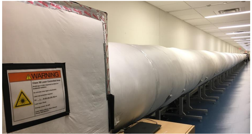
Figure 2: Princeton Starshade Testbed located on campus. This 80 meter long, 1 meter diameter tube provides a clean and dark environment for conducting optical tests on the starshade masks. Data from this experiment are used to validate optical models predicting the starshade's starlight suppression capabilities.
